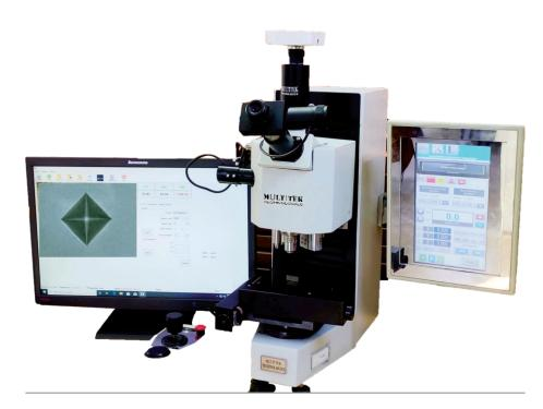
Easy to use motorized stage setup with joystick, touchscreen and software. For easy, accurate and fast testing can be done in any testing process either in manual or auto mode.
